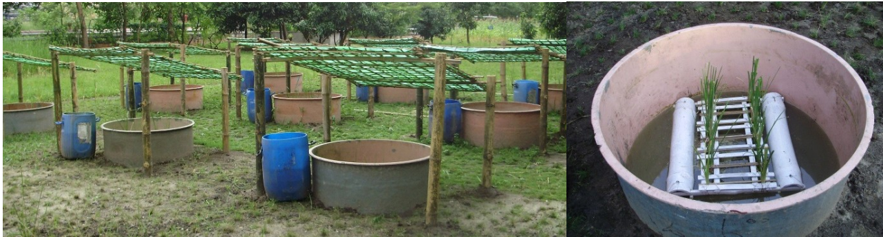
Figure 3: Experimental Tanks for study of hydroponic vetiver
